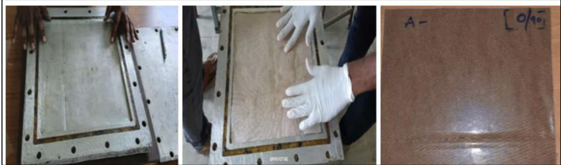
Figure 1: Hand layup process and final specimen
